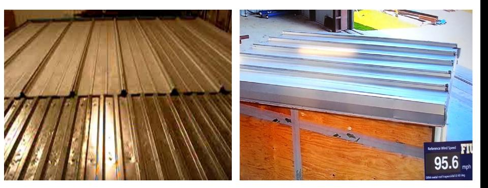
How the broad flat of the panels react to the applied uplift load
