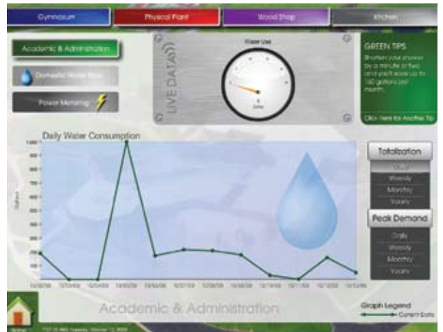
An energy-efficiency education dashboard designed and installed for Chemawa Indian School, in Salem, Ore. The system displays the school's water, power, and gas use on a 19-inch, interactive monitor.
