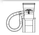
When there is a call for hot water and only three of the eight water heaters fire, a flue check valve eliminates flue gases from entering the water heater cabinet and the building structure. Some are located in the tankless, some use a vent flue check valve adaptors.
