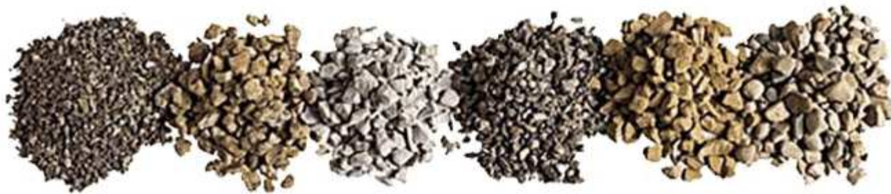
Examples of aggregate fill (from left to right): crushed granite 3/16", decomposed granite 3/8", hard limestone 3/8", carbon canyon 5/16", sanora tan 3/8", sharp angular pea gravel
