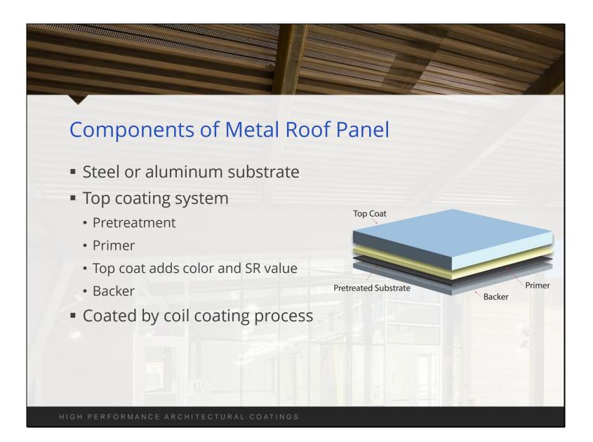
This illustration provides you with an understanding of the coil coating process.
