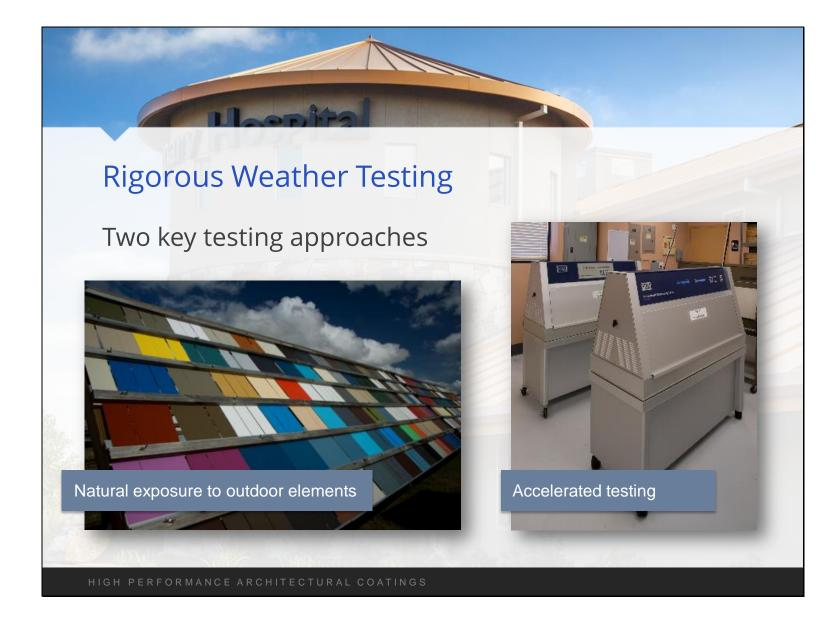
There are a couple of key types of weather testing that are done. The most important and accurate is natural exposure to the elements, which you can see in the photo on the left. This is done at specialty labs in warm climates like Florida, where panels are exposed to high humidity, heat and salt spray...sometimes for decades. This data is crucial to help scientists continue to innovate and improve the performance of coatings.
