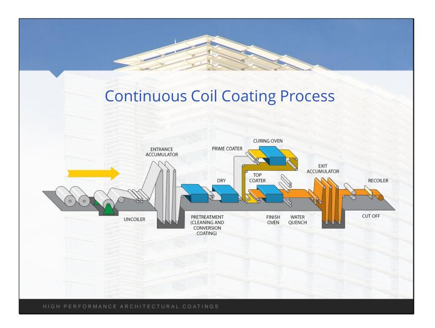
Coil coating lines represent an investment of tens of millions of dollars. On the left you can see the coil being fed into the machine, where it is **Uncoiled.**
