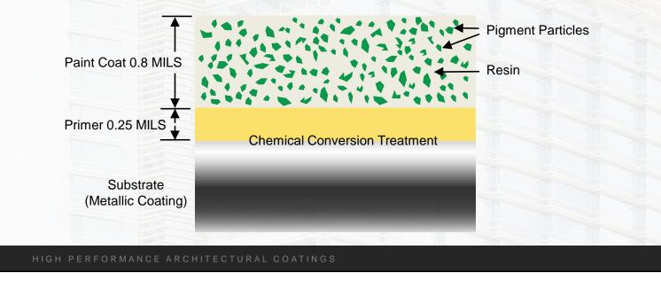
This drawing helps you understand how the coating works to provide protection of the substrate.
