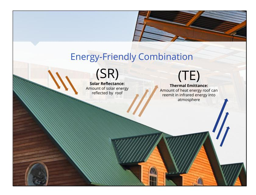
This simple diagram shows the sun hitting the roof and the solar reflective pigments deflecting this thermal energy back to the atmosphere.
