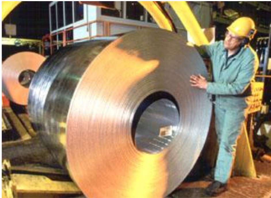
Cold rolled coil is charged into the hot dip line.
