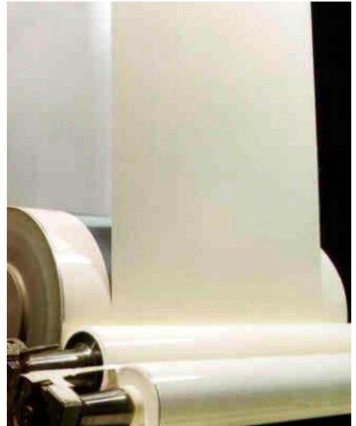
A line coater—a continuous coil coating operation where the coil moves in one direction and the roller in the other to ensure good flow and uniform paint application.
