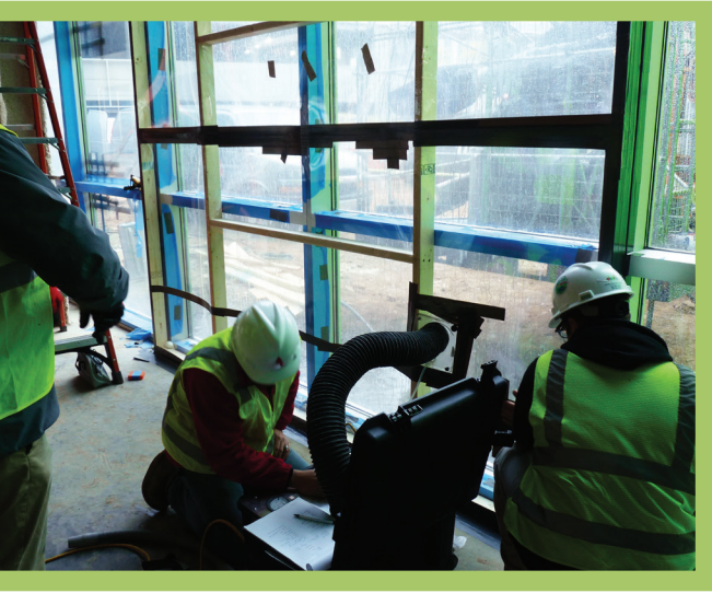
Window performance testing establishes thermal efficiency and moisture protection.
