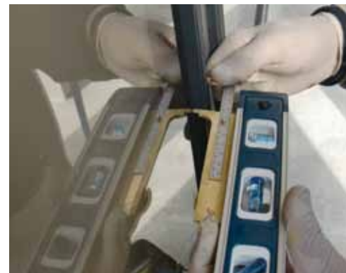
Evaluation may include measurement of gasket hardness (top) and glazing alignment (above). Glazing that exhibits systematic scratches or defects may need to be evaluated for structural integrity under laboratory conditions, the authors warn.
