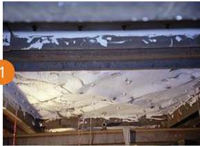
Steel Plate at 5 \delta y (Drift of 3.0%)
